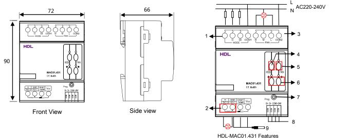
1. Relays I, II and III are used to control air conditioner work mode. These relays can be configured via HDL Buspro software.
