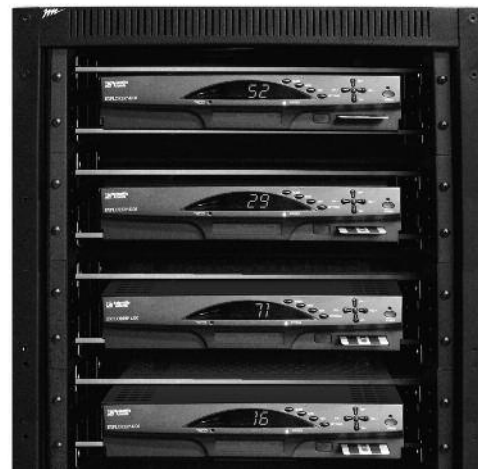
OCAP-3 (shown) uses three space model for greater heat dissipation, use two space model for high density mounting
